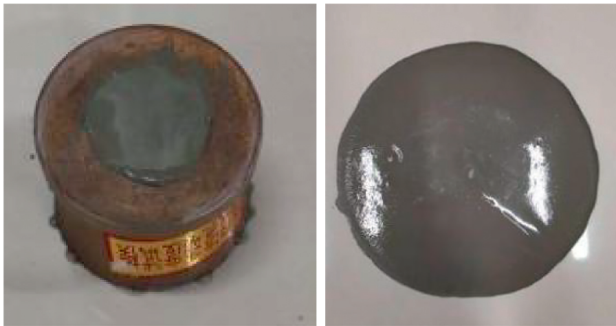
FIGURE 2: The test of material fluidity.
