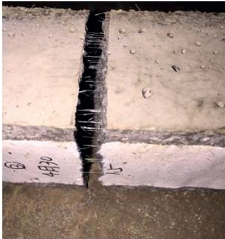
FIGURE 5: Flexural fracture of CGA mortar.
