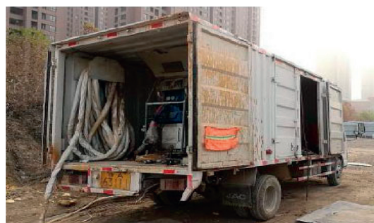
FIGURE 5: Vehicle-mounted polymer grouting integrated system.
