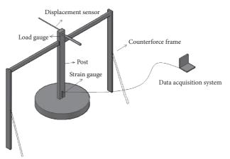
FIGURE 3: Schematic diagram of the loading system.
