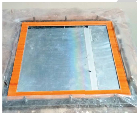
FIGURE 5: Aluminum sheets used for curing for smooth finishing.
