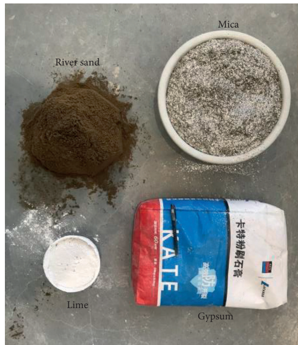
FIGURE 10: Schematic diagram of raw materials for the similar simulation test.
