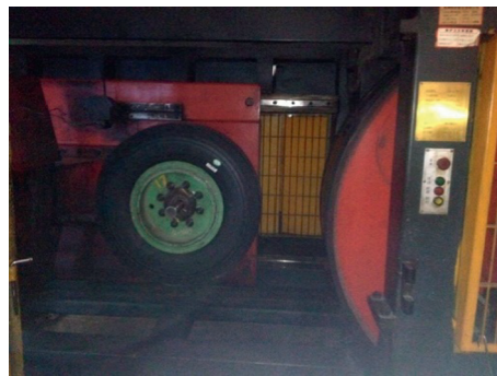
FIGURE 2: Real fatigue test stand with a tire.
