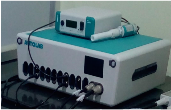
FIGURE 1: Electrochemical workstation to identify the utilization of potentiodynamic polarizing bends and electrochemical impedance spectroscopy.
