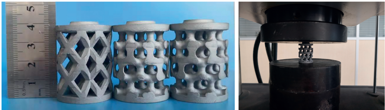
FIGURE 14: Specimens with AM and their compression test.
