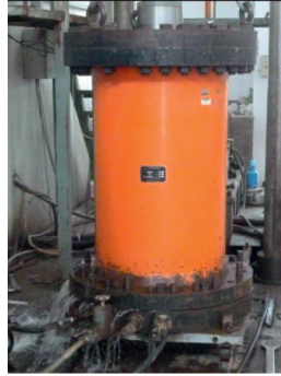
FIGURE 2: TYD-1500 dynamic triaxial tester.
