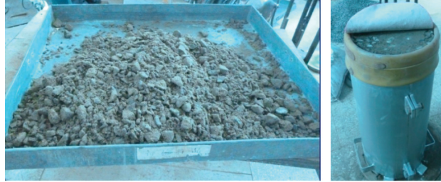
FIGURE 1: The specimen of LCSG material for the triaxial test.
