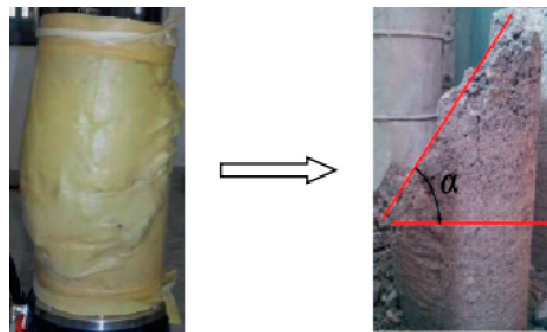
FIGURE 5: The final failure modes of specimens for LCSG material.
