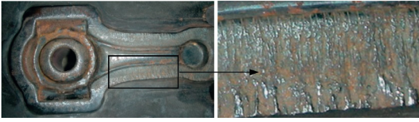
FIGURE 1: Hot die forging of the connecting rod and detail of the surface of the used H13 forging die showing severe plastic deformation.
