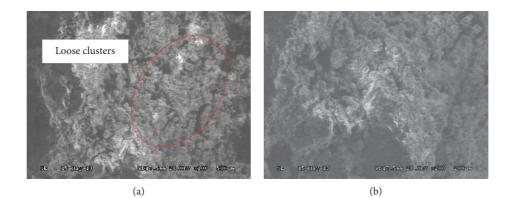
FIGURE 6: SEM picture of coal body: (a) 100 times; (b) 200 times.
