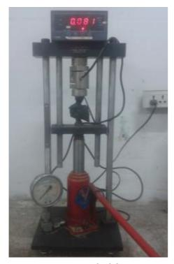
FIGURE 2: Point-load device.
