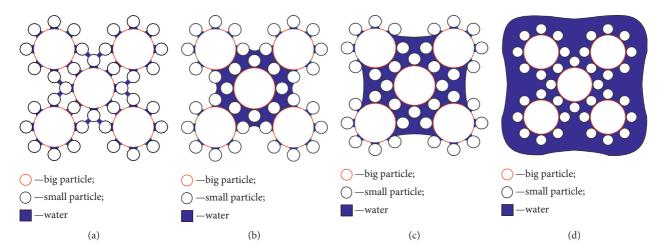
FIGURE 9: Shape of water-coal liquid bridge at different stages: (a) State II; (b) State II; (c) State III; (d) State IV.
