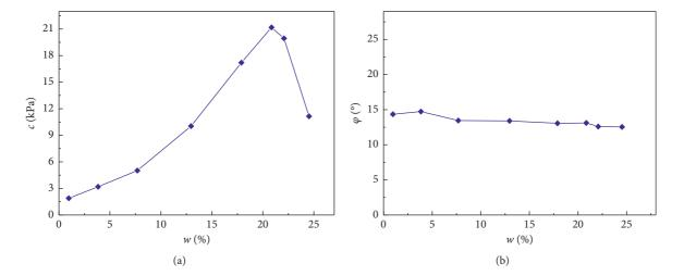
FIGURE 8: Cohesion (a) and internal friction angle (b) of coal under different water contents.
