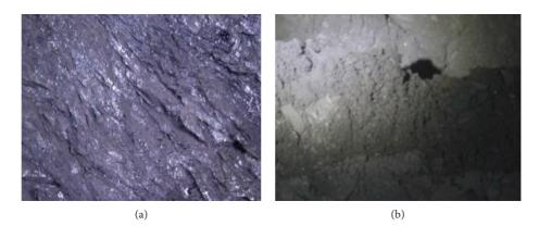
FIGURE 1: State of coal seam: (a) coal wall; (b) dropped loose coal.
