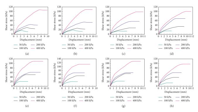
FIGURE 7: Shear stress-displacement curve of extremely soft coal: (a) w = 0.966%; (b) w = 3.841%; (c) w = 7.688%; (d) w = 12.957%; (e) w = 17.888%; (f) w = 20.847%; (g) w = 22.072%; (h) w = 24.526%.
