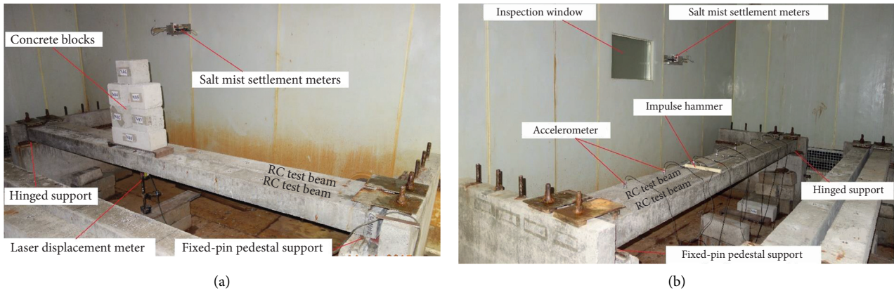
FIGURE 2: Experimental layout in the marine environmental chamber: (a) static test and (b) dynamic test.
