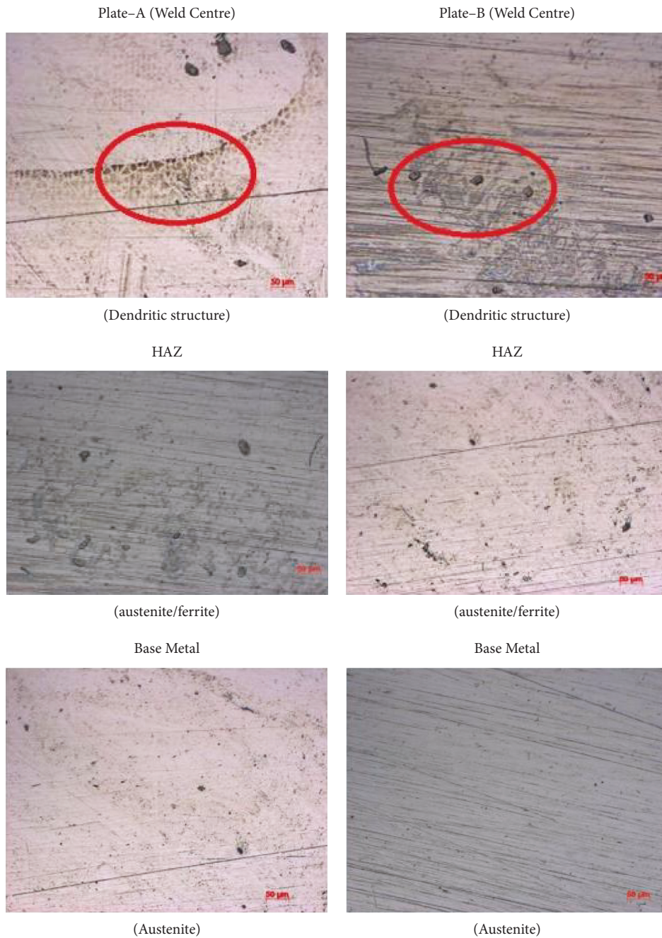
FIGURE 13: Microstructure analysis of welded specimens.
