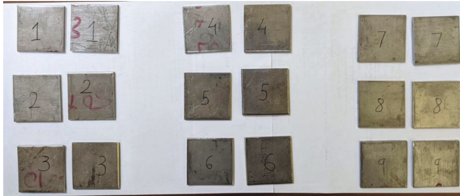
FIGURE 1: 9 pairs of 310 SS sheet specimen before welding (base metal).
