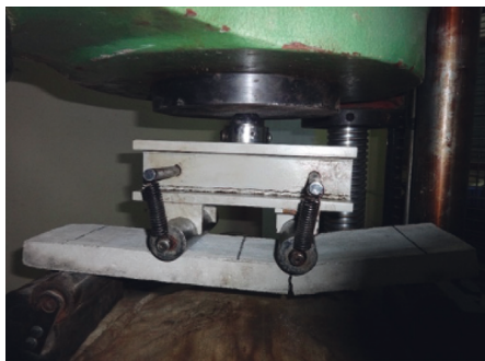
Formation of cracks in panels tested under flexure
