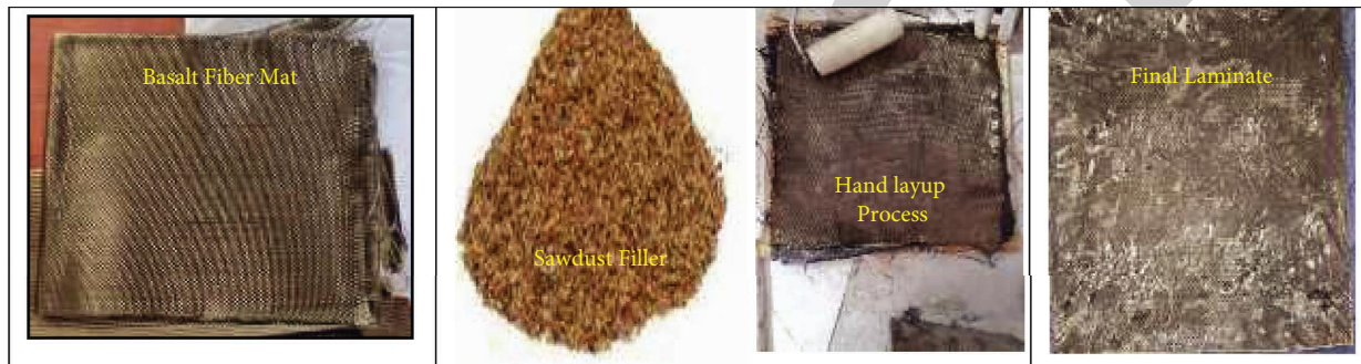
FIGURE 2: Fabrication process of basalt fiber composite.
