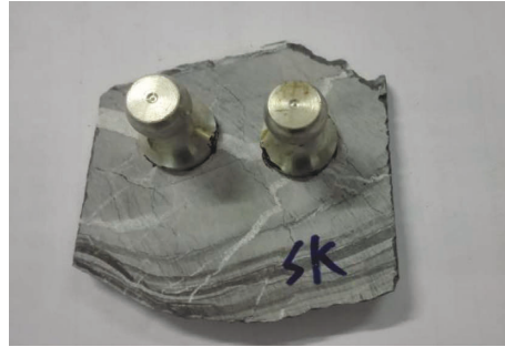
FIGURE 4: Specimen for bond strength test.
