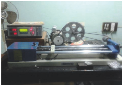
FIGURE 3: Tensile test-digital tensometer setup.
