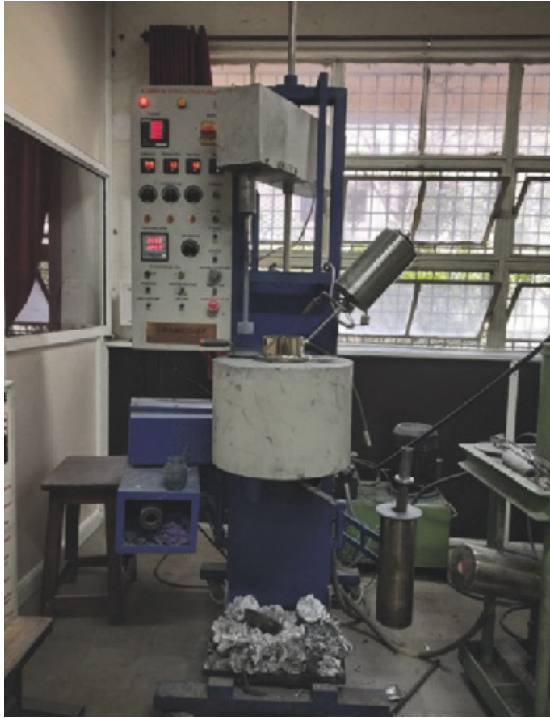
FIGURE 2: Experimental setup of the stir casting process.
