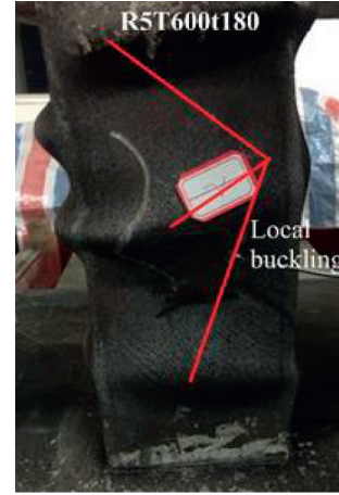
FIGURE 3: The typical failure mode of tested specimen.
