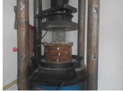
FIGURE 2: ARGFRC compression test.
