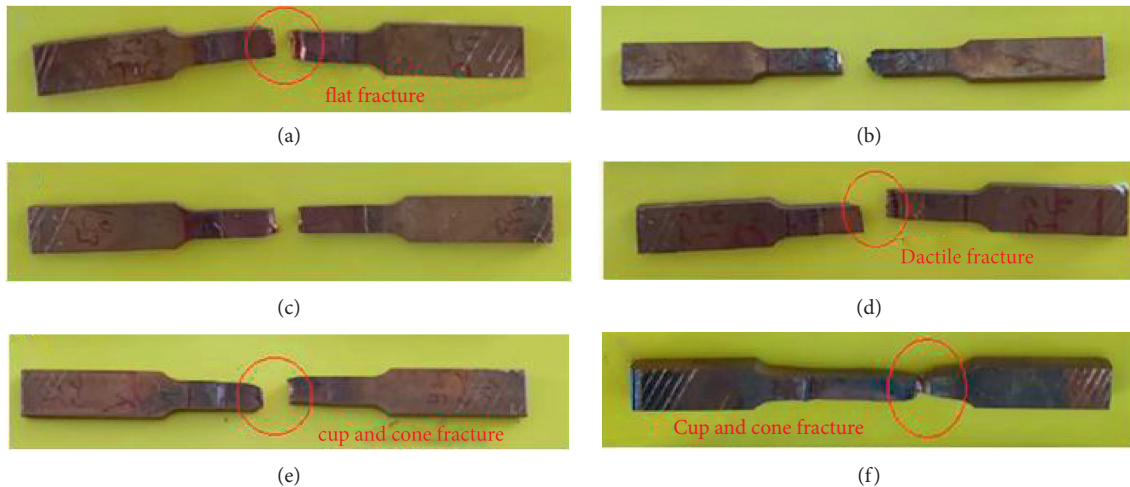
FIGURE 3: Fractured tensile samples.
