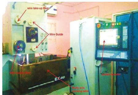
FIGURE 4: Wire cut EDM machine setup.
