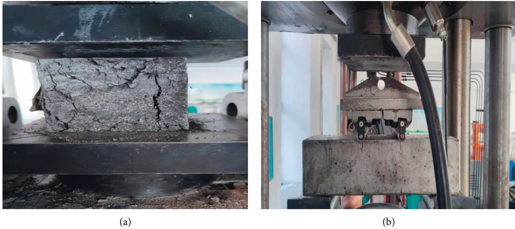
FIGURE 1: (a) Compressive strength tests. (b) Flexural strength tests.
