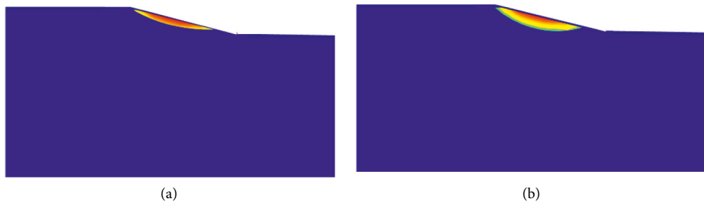
FIGURE 8: Stability analysis of potential sliding surface of slope. (a) Rain strength 38.8 mm/d. (b) Rain strength 77.6 mm/d.
