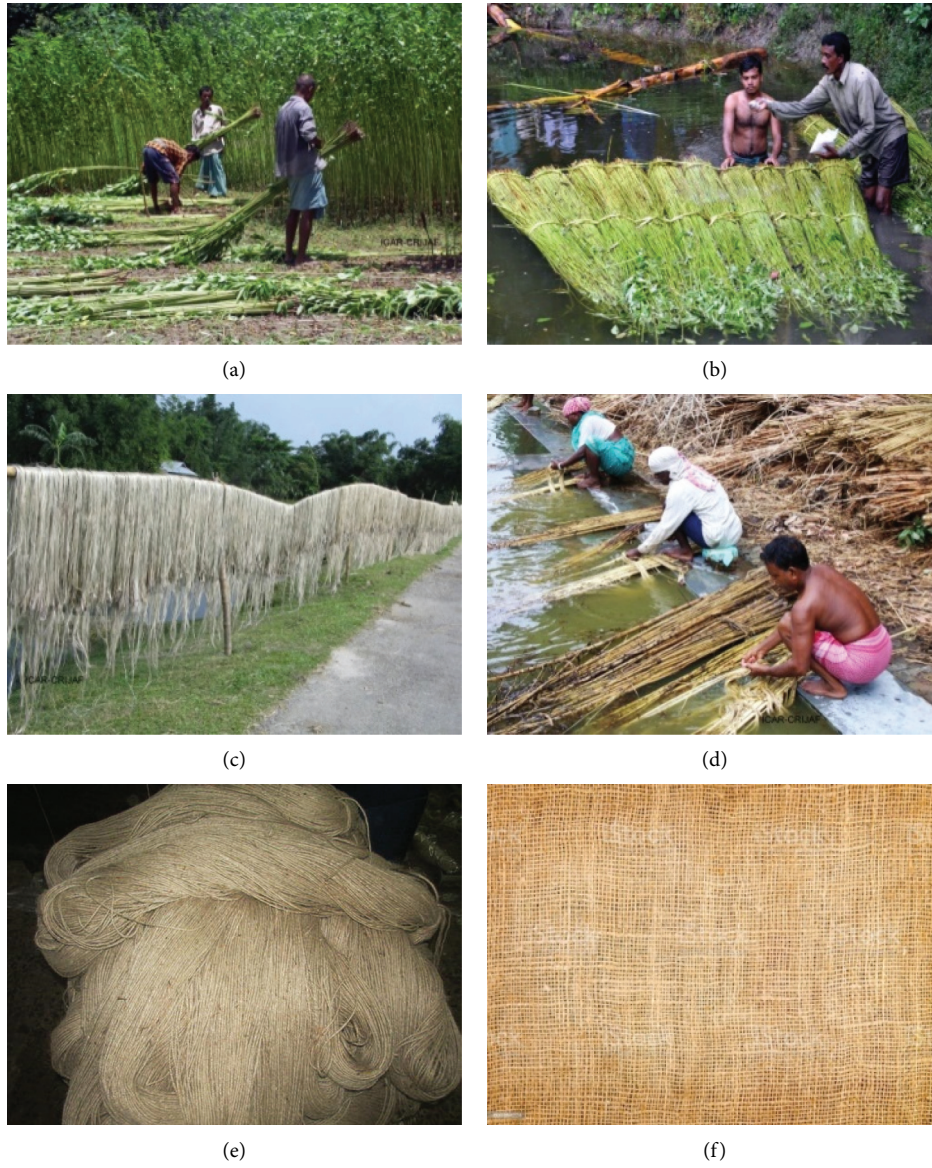
FIGURE 1: Process of jute fibres to jute fabric. (a) Bundle stalk. (b) Retting. (c) Sundry. (d) Strapping and washing. (e) Jute yarn. (f) Jute sack.
