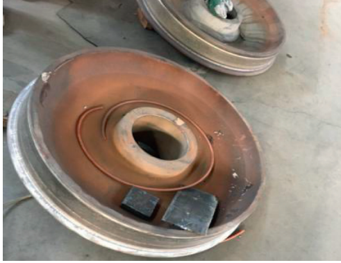
FIGURE 2: Wheel remanufactured using laser cladding.
