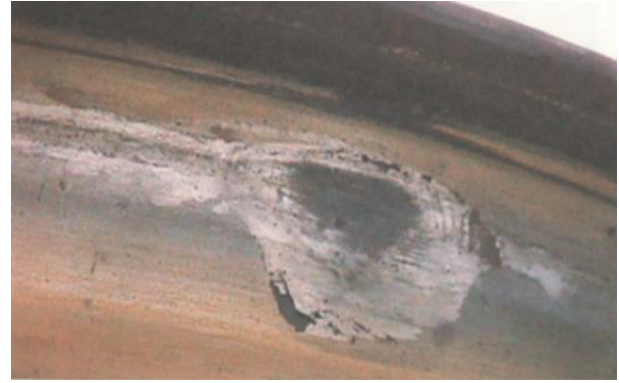
FIGURE 1: Wheel tread abrasion.
