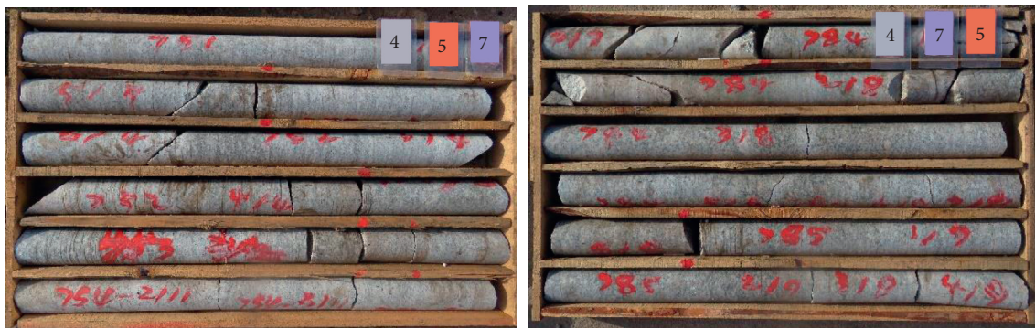
FIGURE 3: Core exposure of some strata (-1815.56~-1820.16 m, -1897.46~-1902.06 m).
