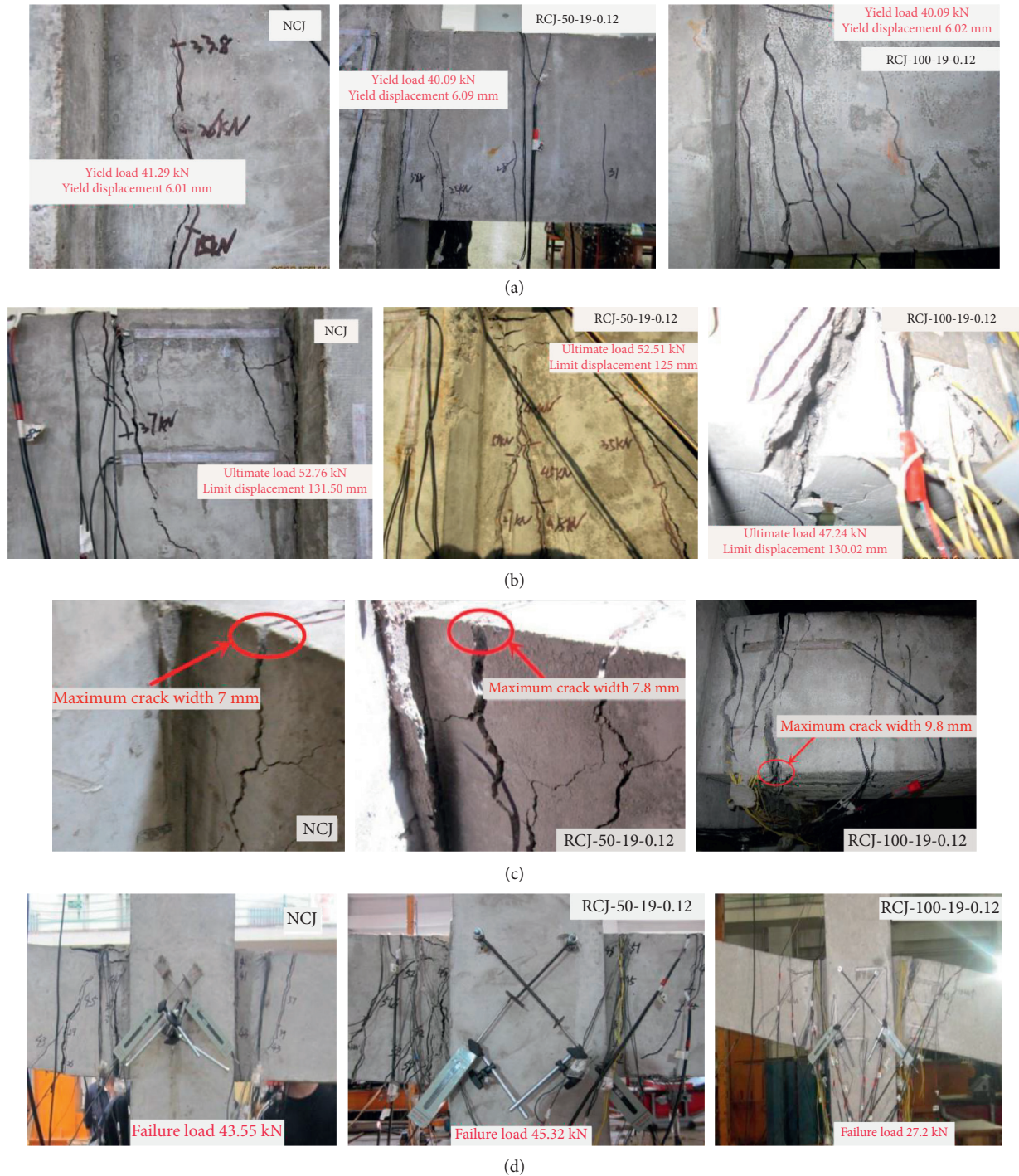
FIGURE 7: Experimental phenomena. (a) Yielding stage. (b) Ultimate stage. (c) Maximum crack width of beam end. (d) Joint form under failure load.
