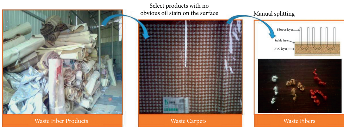
FIGURE 2: The preparation of waste fibers.
