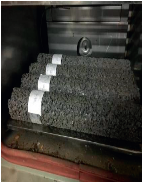
FIGURE 4: Specimens in the freeze-thaw chamber.
