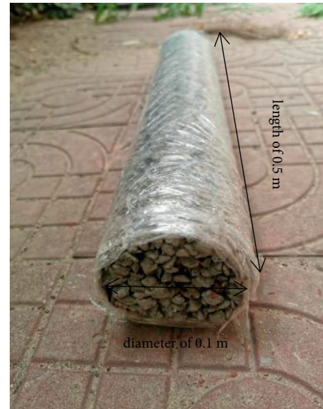
FIGURE 2: Seepage well wrapped in plastic film.
