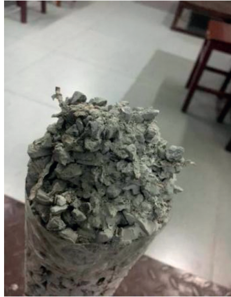
FIGURE 6: The damaged specimen in the compression test.
