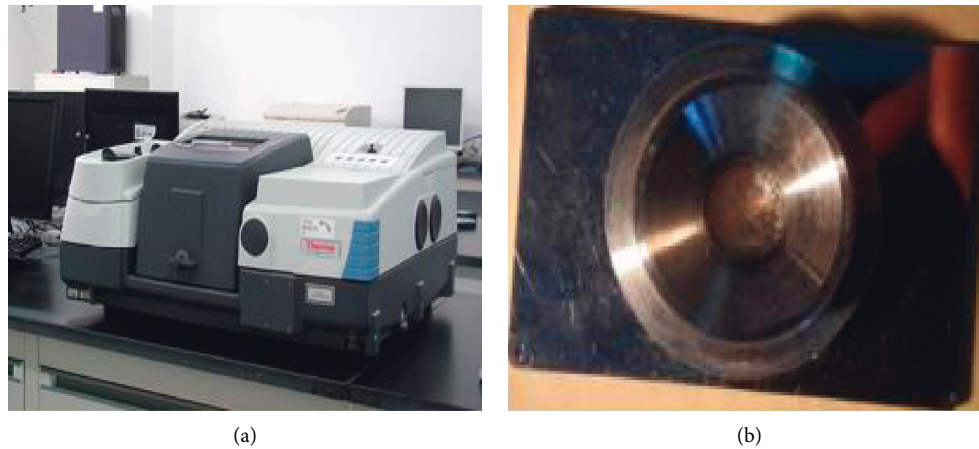
FIGURE 5: Fourier transform infrared spectrometer characterization: (a) the equipment and (b) test sample.
