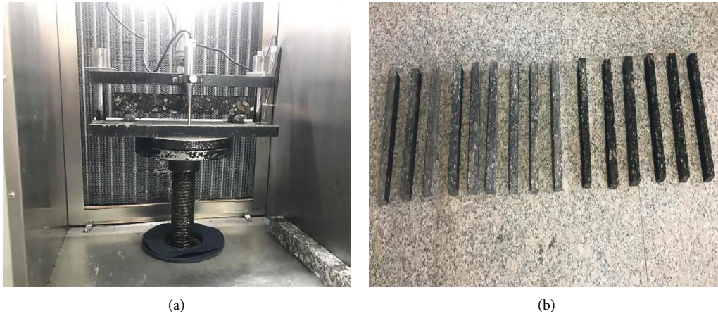
FIGURE 7: Asphalt mixture low-temperature bending test: (a) the equipment and (b) test sample.
