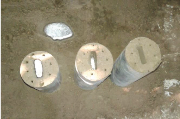
FIGURE 2: Poured molten metals into die.
