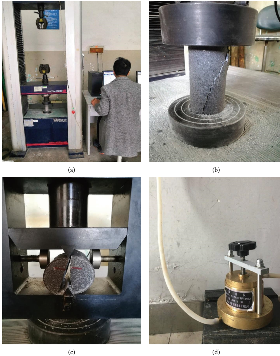
FIGURE 3: Process of testing analogous materials. (a) Uniaxial compression test; (b) failed specimen after compression; (c) brazilian splitting test; (d) permeability test.
