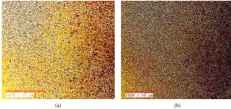
FIGURE 5: Microstructure of the NZ (a) at 0^\circ tool angle and (b) at 1.5^\circ tool angle.
