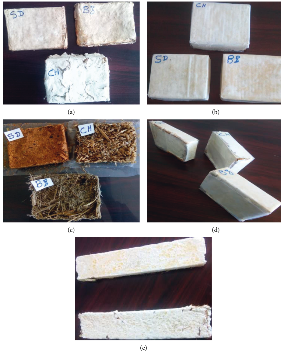
FIGURE 4: Image showing Mycoblock made from different substrates: (a) heat exposed, (b) nonheat exposed, (c) control, (d) block side view, and (e) rectangular sheets.
