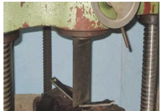
FIGURE 4: Flexural testing of the specimen sample.
