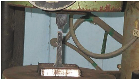
FIGURE 3: UTM tensile testing of the sample specimen.
