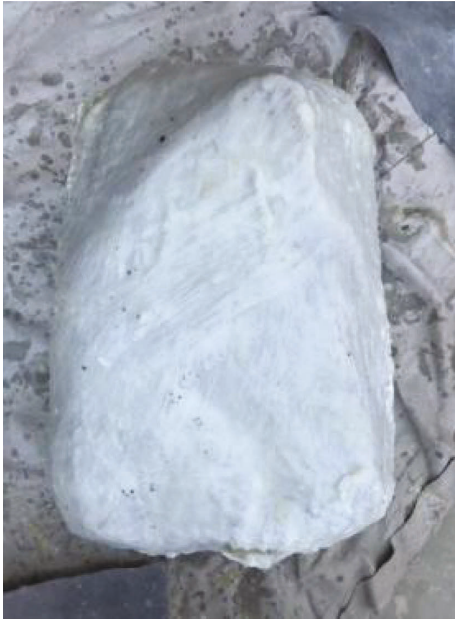
FIGURE 1: Sealing and preservation of the rock block with wax.
