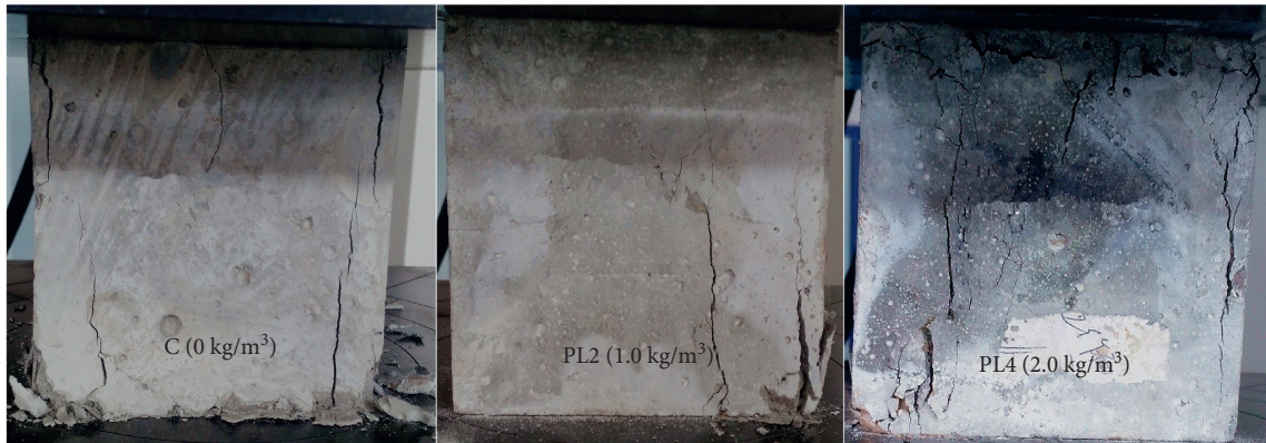
FIGURE 4: Failure mode of compression specimen.
