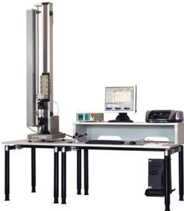
FIGURE 8: Multipurpose microtensile testing machine.
