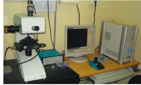
FIGURE 5: Microhardness tester (UHL VMHT digital).
