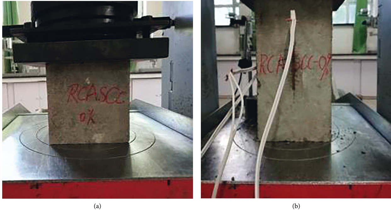
FIGURE 7: Process of compression tests. (a) Cube compression test. (b) Prism compression test.
