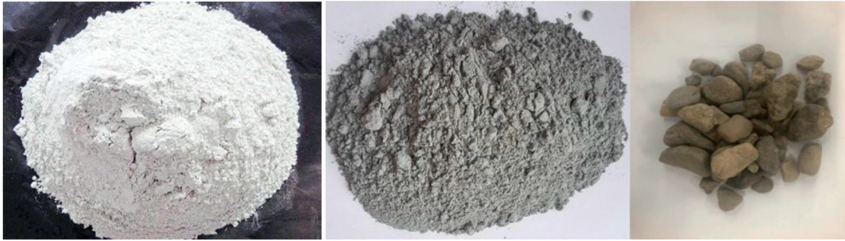
FIGURE 1: Slag powder, fly ash, and large size cobbles.
