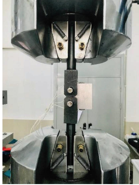
FIGURE 4: CT specimen mounted in a fatigue machine.
