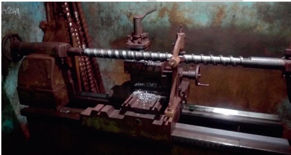
FIGURE 9: Machining image of single screw conveyor.
