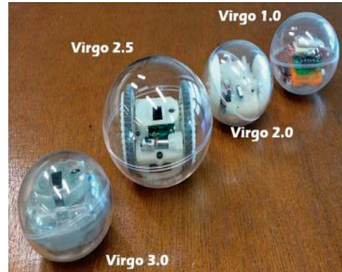
FIGURE 1: Spherical robot (VIRGO) [5].
