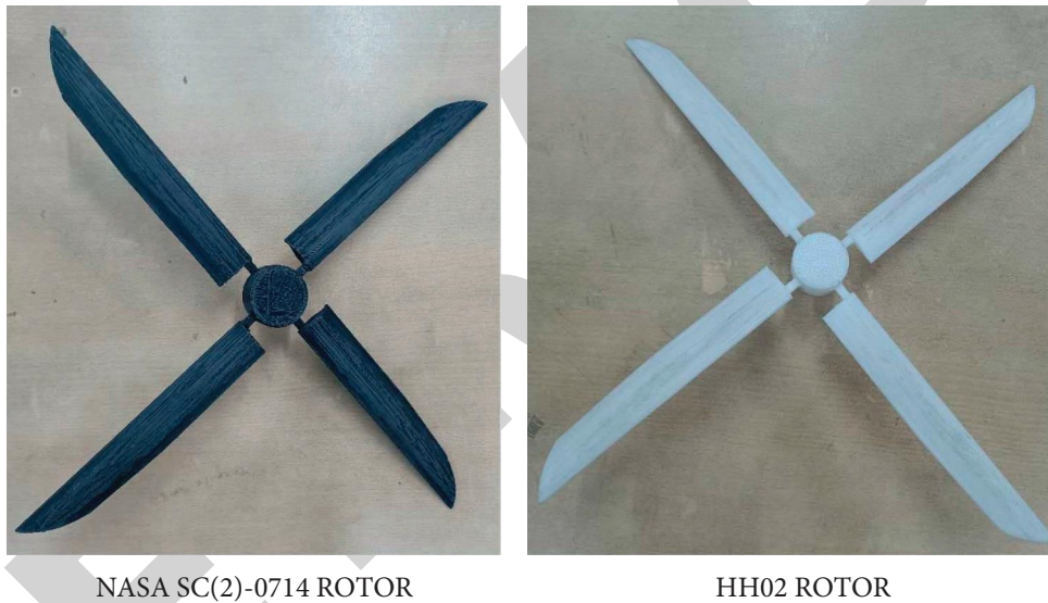
FIGURE 6: 3D printed models used for testing.
