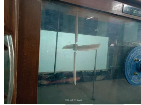
FIGURE 7: HH02 rotor model in the wind tunnel.
