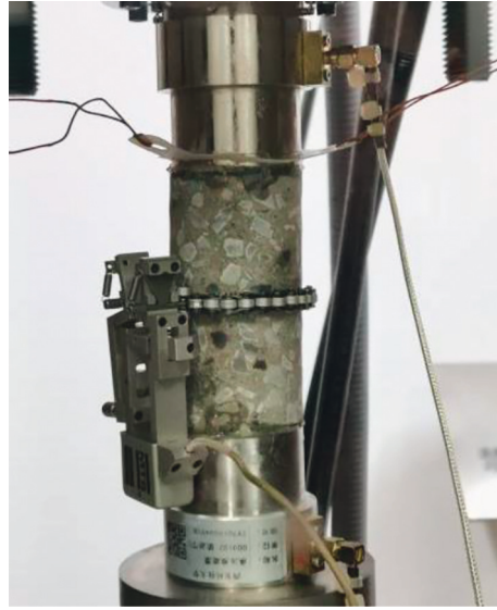
FIGURE 2: Uniaxial loading of concrete sample.
