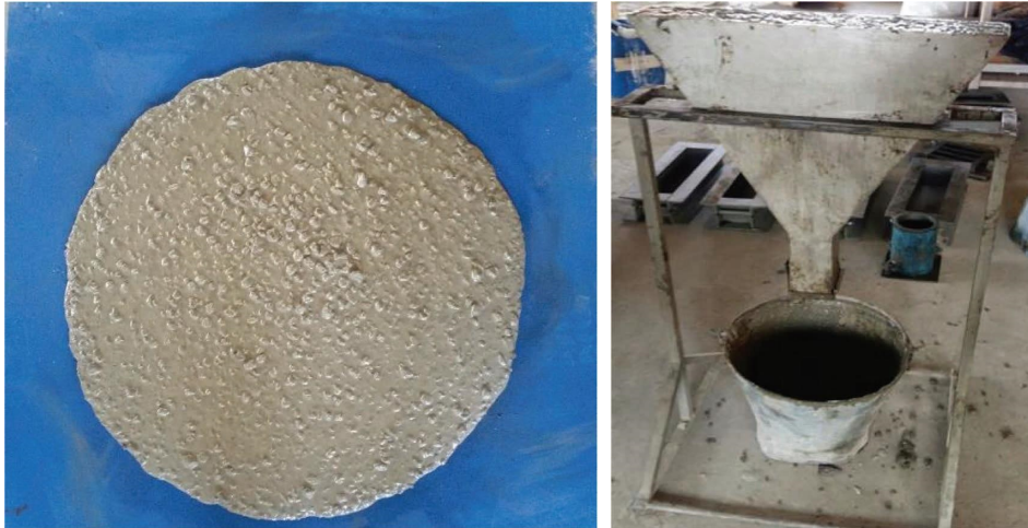
FIGURE 2: Standard slump cone test and V-funnel test.
