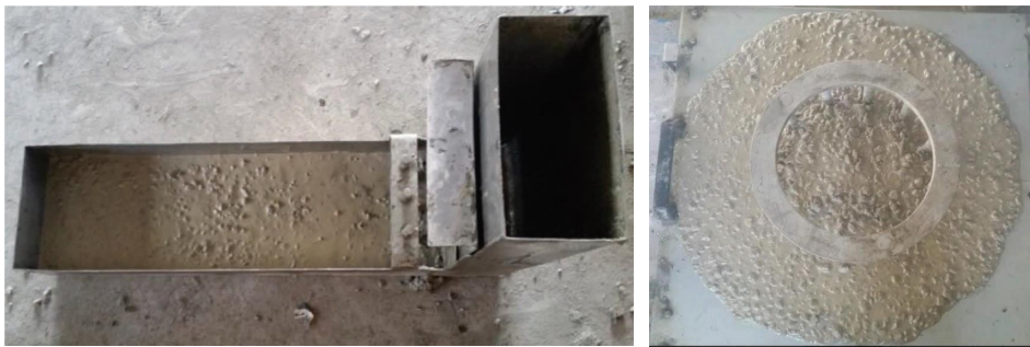
FIGURE 3: L-box test and J-ring test.
