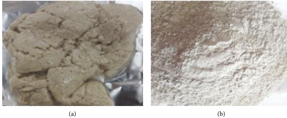
FIGURE 2: (a) Precipitated protein and (b) powder keratin after freeze-drying and grinding.
