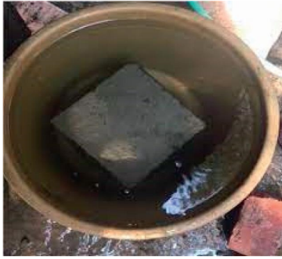
FIGURE 6: Specimen immersed in H_2SO_4 .
