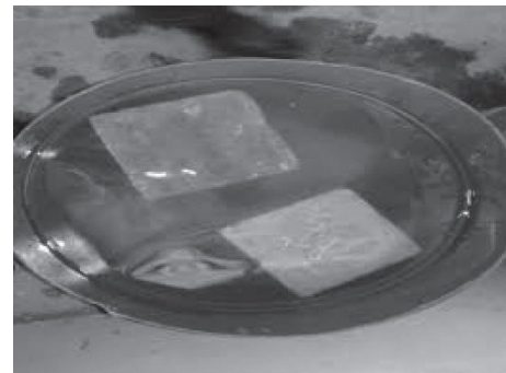
FIGURE 5: Specimen immersed in Hcl.
