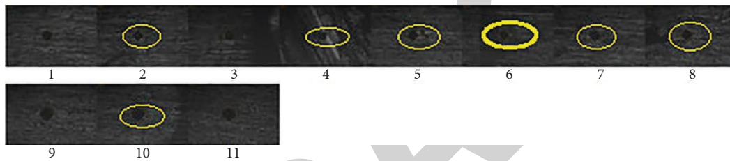
FIGURE 16: Vickers microhardness indentations: (Cu-AS) side: points 1-3 base metal area, points 3-6 HAZ and TMAZ, point 6 Al-Cu interface area (weld joint area), (Al-RS) side: points 6-9 TMAZ and HAZ, and points 9-11 base metal area (Al).
