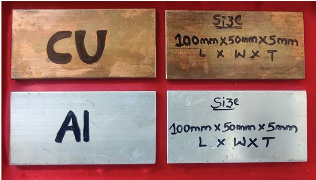
FIGURE 4: Crafted plates of C11000 and AA6101.
