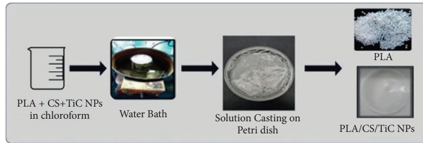
FIGURE 1: Synthesis of poly(lactic acid)/chitosan/titanium carbide nanoparticles.
